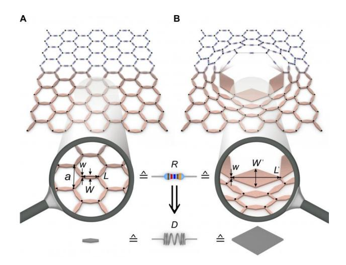
Mechanical cloak of invisibility: In a regular honeycomb structure (left), a hole is compensated by a distortion (right). External forces act as if the hole would not exist. Credit: T. Bückmann/KIT
