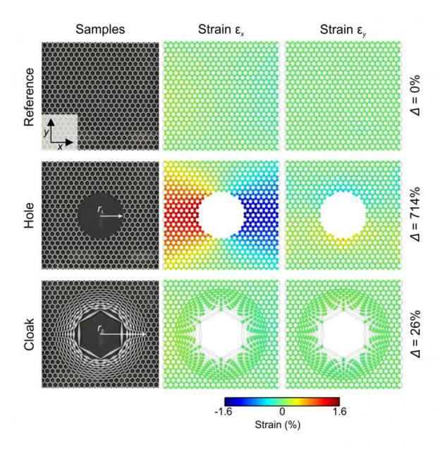
Analysis of a hole in a hexagonal structure: External forces strongly deform the structure, the structure is unstable. By means of the new construction method,
