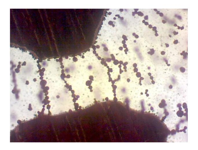
This screenshot from the video below shows the self-healing of an open circuit fault. When a fault occurs, an electric field develops in the gap, which polarizes the conductive particles in the fluid. The positively charged end of each polarized particle aligns with the negatively charged end of another particle due to dipole interactions, causing the particles to form a bridge between the two electrodes. Credit: Nair, et al. ©2015 AIP Publishing
