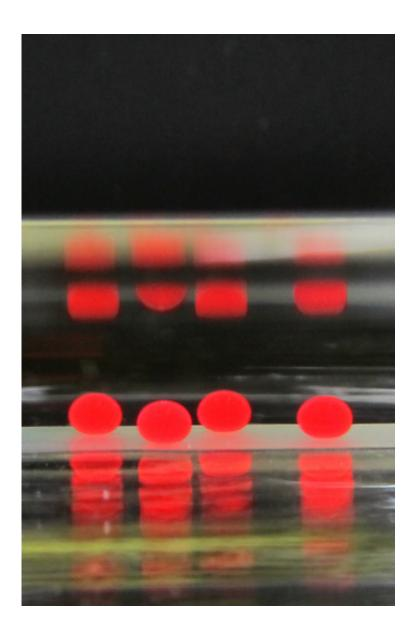
Droplets of oil resting above a superoleophobic surface. Because of the material's oil-repelling qualities, the drops essentially remain suspended above
