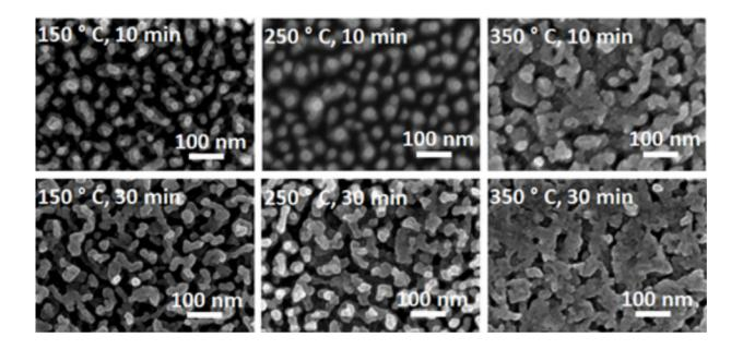
Growth of nanostructures on a copper surface at different temperatures and exposure times. Credit: Tanyeli et al. / Nature Scientific Reports
