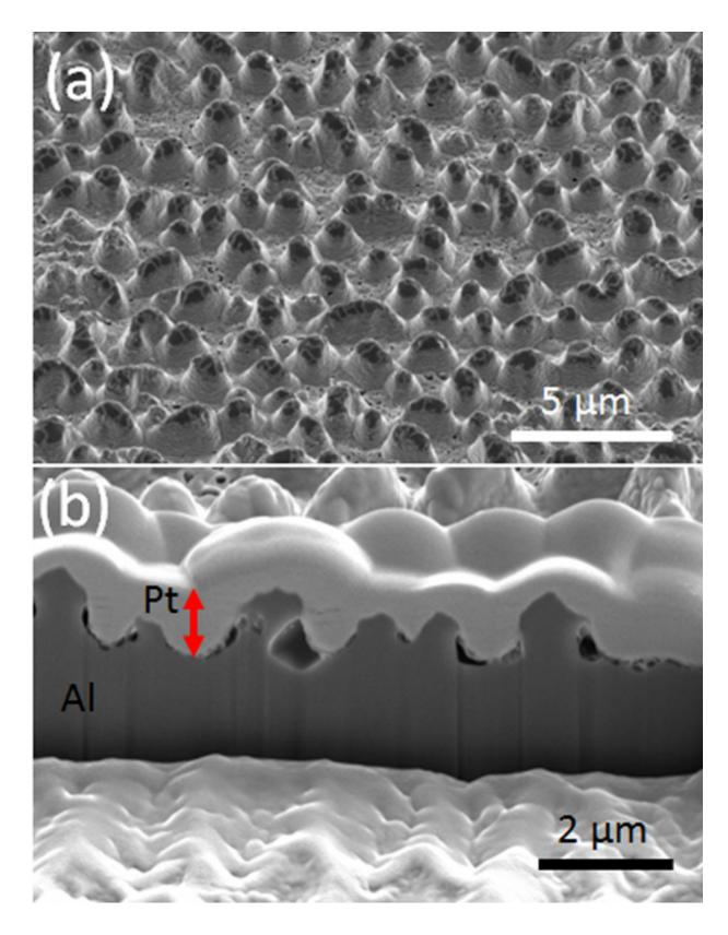
Overview (a) and cross-section (b) of nanostructures on an aluminium surface.
