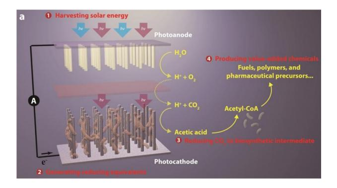
This break-through artificial photosynthesis systems has four general components: (1) harvesting solar energy, (2) generating reducing equivalents, (3) reducing CO2 to biosynthetic intermediates, and (4) producing value-added chemicals. Credit: Berkeley Lab
