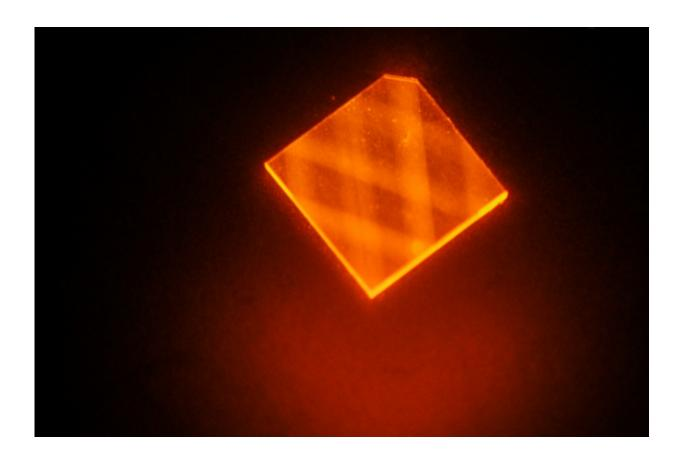
In this image, laser light enters a synthetic diamond from a facet at its corner and bounces around inside the diamond until its energy is exhausted. This excites "nitrogen vacancies" that can be used to measure magnetic fields. Credit: H. Clevenson/MIT Lincoln Laboratory
