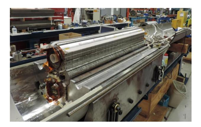
This magnet recently achieved an important milestone, reaching its design field of 11.5 Tesla. It is the first successful niobium-3-tin, twin-aperture accelerator magnet in the world. Credit: Sean Johnson, TD
