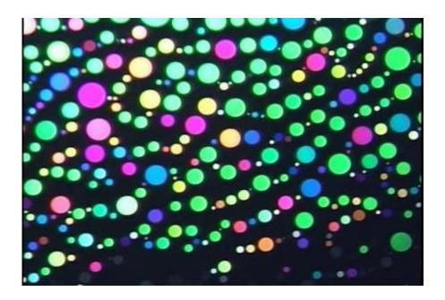
Microscopic detail of liquid crystal islands tethered like necklaces when an external electric field is applied near the very thin film surface. Credit: Liquid Crystal Physics Group/University of Colorado Boulder
