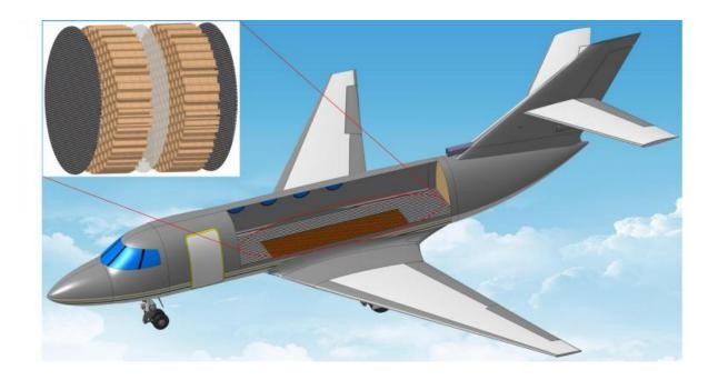
Researchers have developed membranes that can significantly reduce aircraft noise when inserted into the honeycomb structures used in aircraft design. Credit: Yun Jing, North Carolina State University
