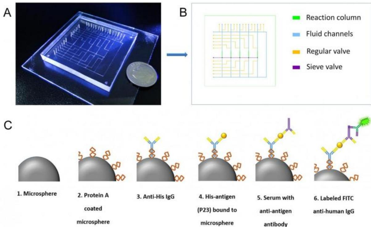
Microfluidic chip, with a diagram of its channels and antigen-labeling process.
