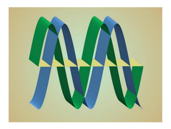
Schematic image indicating the inferred intertwining of the superconducting wave function (green) with the envelope function (blue) for the atomic magnetism. The amplitudes of both functions oscillate in space to positive and negative values about the zero-amplitude plane (yellow). Note, the maximum of one function occurs where the other passes through zero. The relative shift between the two functions minimizes their overlap. Credit: Brookhaven National
