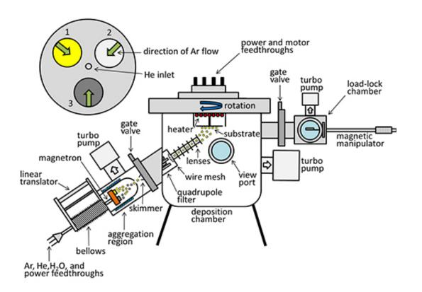
Scientists at Pacific Northwest National Laboratory created metal alloy particles using a technique that involves magnetron sputtering and gas aggregation. They placed them on a surface using ion soft landing techniques. Credit: Johnson et al. with permission from the Royal Society of Chemistry.
