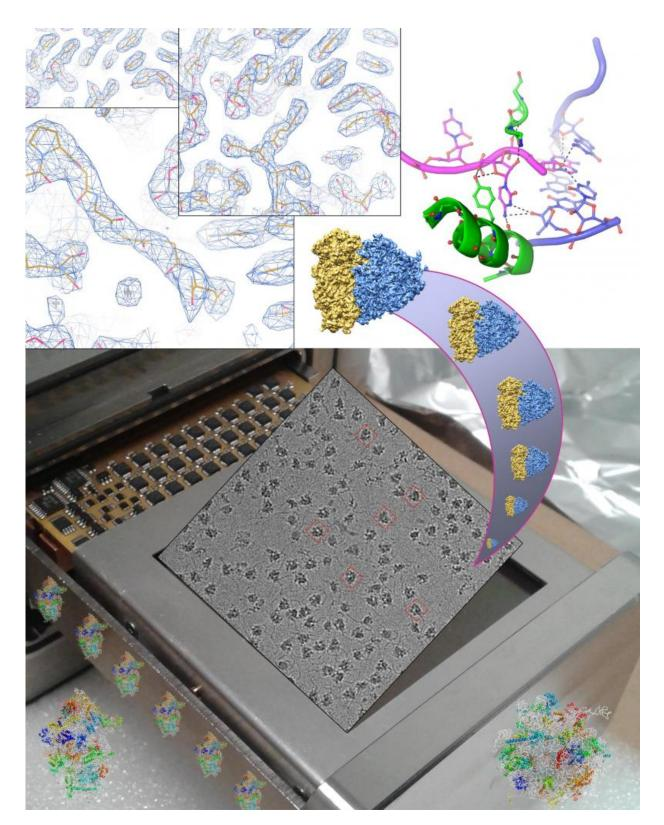
3D atomic reconstruction from high-resolution images obtained with a cryoelectron microscope using a highly sensitive direct electron detection camera.
