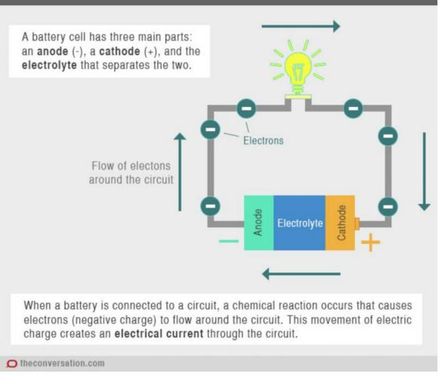
Because lithium has a strong electrochemical driving force to be oxidised if allowed, it migrates back to the cathode to become a Li+ ion again and gives up its electron back to the cobalt ion. The movement of electrons in the circuit gives us a current that we can use.
