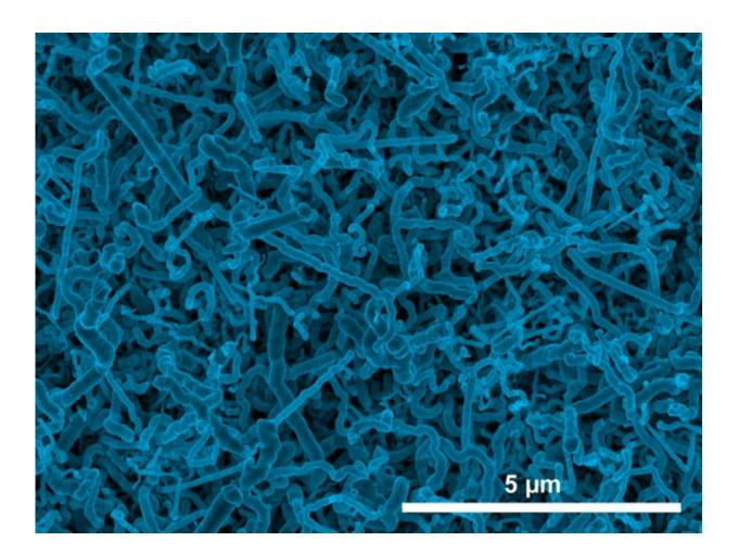
Scanning electron micrograph image of germanium nanowires electrodeposited onto an indium tin oxide electrode from aqueous solution. Credit: Jay Switzer
