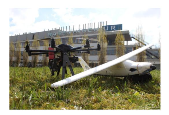
Unmanned aircraft are creating new opportunities for scientific research. A fixed wing airplane, for example, can be used to compile detailed 3D models of a specific area for research into erosion, or to map larger areas. An octocopter can help with research into precision farming, vegetation or forests, for example, and can be used to survey specific marine areas, such as coral reefs. Aerial research using these aircraft has
