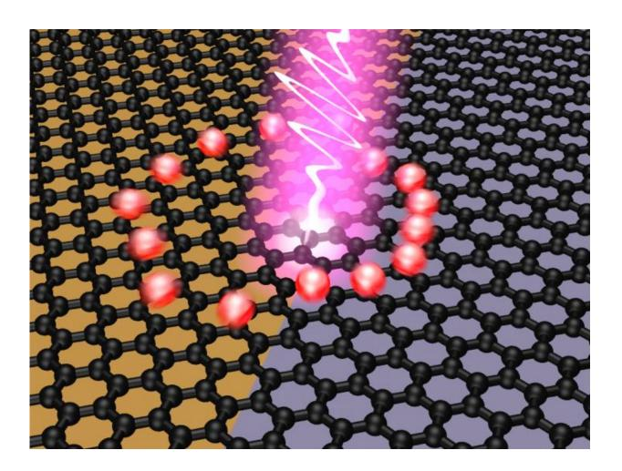
This is an illustration of ultrafast photovoltage creation after light absorption at the interface of two graphene areas with different Fermi energy. Credit: ICFO/Achim Woessner.
