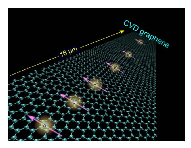
In graphene, electrons keep their magnetization, their spin (the pink arrows in the picture) much longer than they do in ordinary conductors such as copper and aluminum. This characteristic of graphene may enable spintronics to become a complement to traditional electronics, which only utilizes one of the electron's degrees of freedom, namely their charge. Credit: M Venkata Kamalakar et al, *Nature Communications*
