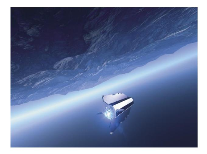
Along with its sleek design, the gravity-mapping GOCE mission achieved dragfree flight with an electric ion propulsion system mounted at the back of the satellite. Unlike conventional engines, it used electrically-charged xenon to create a gentle thrust. The system continually generated tiny forces to counteract the drag the satellite experienced as it cut through the remnants of Earth's
