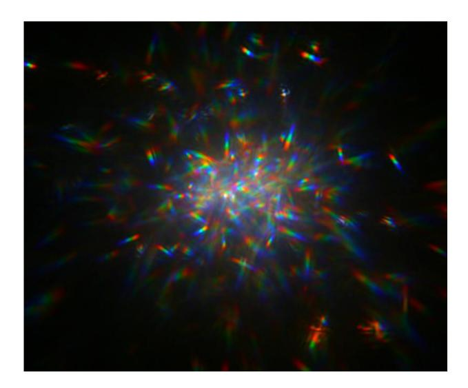
This image shows laser light reflected off of a glitter mirror onto a camera sensor. Researchers tested this in a laboratory as part of the concept of "Orbiting Rainbows," a low-cost solution for space telescope mirrors. Credit: G. Swartzlander/Rochester Institute of Technology
