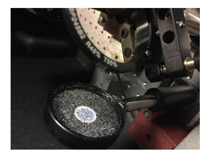
Researchers made a mirror surface out of glitter to test the idea of using a cloud of reflective particles as a space telescope mirror. They took images of two light sources using this mirror in a laboratory at Rochester Institute of Technology. Credit: G. Swartzlander/Rochester Institute of Technology
