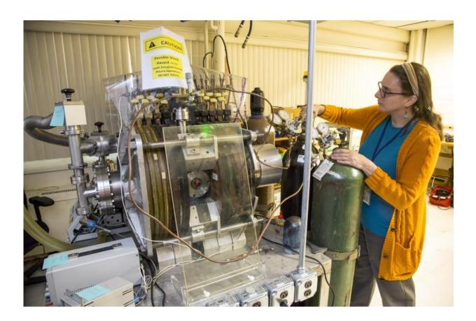
Lenore Rasmussen, Ph.D., principal investigator of the Synthetic Muscle investigation, checks the pressure during the oxygen plasma treatment of titanium metal support mounts at the US Department of Energy's Princeton Plasma Physics Laboratory. Credit: Elle Starkman, PPPL
