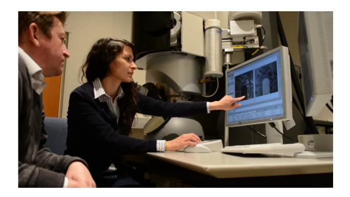
PNNL scientists Nigel Browning and Layla Mehdi examine images from a scanning transmission electron microscope outfitted with a battery cell stage that lets them view multiple cycles of rechargeable battery use under real-world conditions.
