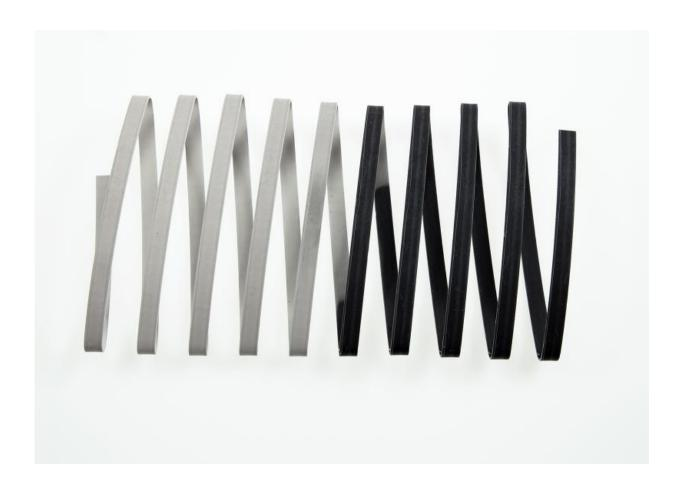
Metal strip coated with thermochromic nanoparticles. At temperatures above 30° Celsius (about 86 °F), the coating is transparent and the metal underneath reflects heat. Credit: Fraunhofer ICT
