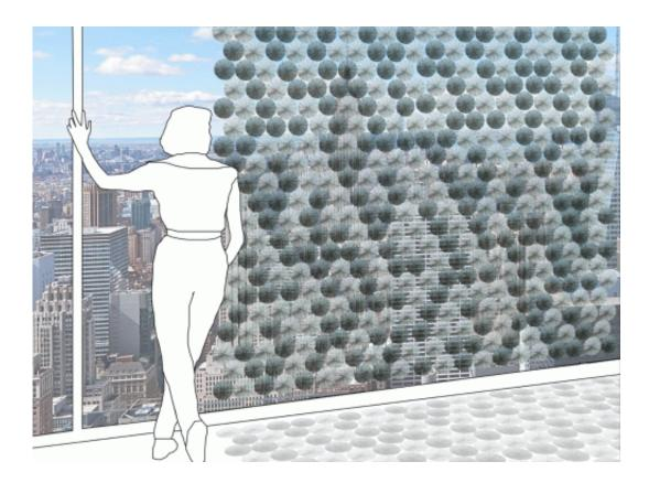
The façade element operates using integrated shape-memory alloys and so doesn't require an external power source. Credit: Bára Finnsdóttir | Weißensee School of Art Berlin
