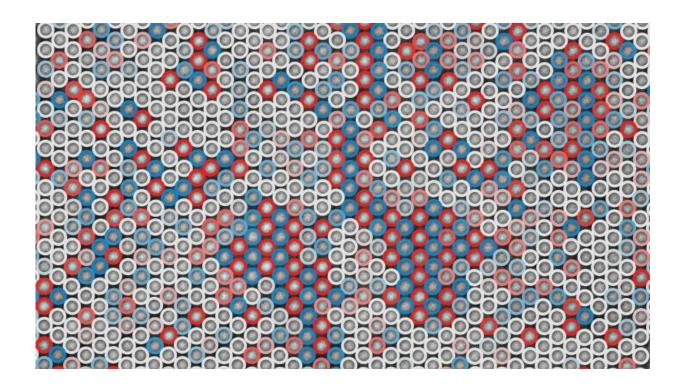
Scanning transmission microscopy image with intensity ratios highlighted. The ordered nano domains have columns with higher intensity (red) residing next to columns of lower intensity (blue). Credit: Doug Irving and James LeBeau, North Carolina State University
