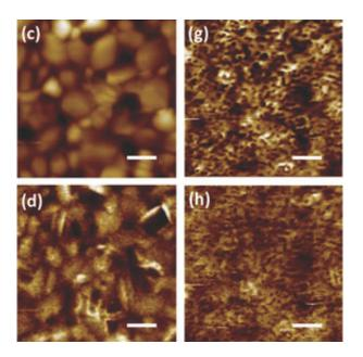
Height (c) and photothermal induced resonance (d) images of a sample area before annealing, and the same sample area after annealing 60 min (g,h). Scale bars are 1 micrometer. Data that the group gathered suggest that during curing, metal ion clusters are left on the OTP film surface. These ion clusters could act as charge traps, enabling the material's increased sensitivity. Credit: NIST
