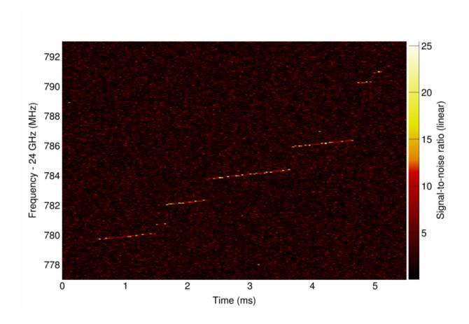
This spectrogram shows the first electron detected by the Project 8 collaboration. The horizontal axis is time, the vertical axis is frequency, and the color is power. Multiple separate "tracks" are seen because the electron scatters off of gas molecules and ends up emitting cyclotron radiation at slightly different frequencies; the slope of each track indicates that the electron is losing energy to the cyclotron radiation.
