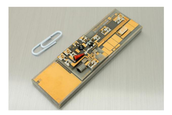
Micro-integrated Extended Cavity Diode Laser (ECDL) for laser spectroscopy of rubidium atoms in space. This module has been used on April 23 for tests on board the FOKUS research rocket aiming to demonstrate whether there really are no differences in how clocks run differently under space conditions like Einstein claimed. Credit: FBH/P.Immerz
