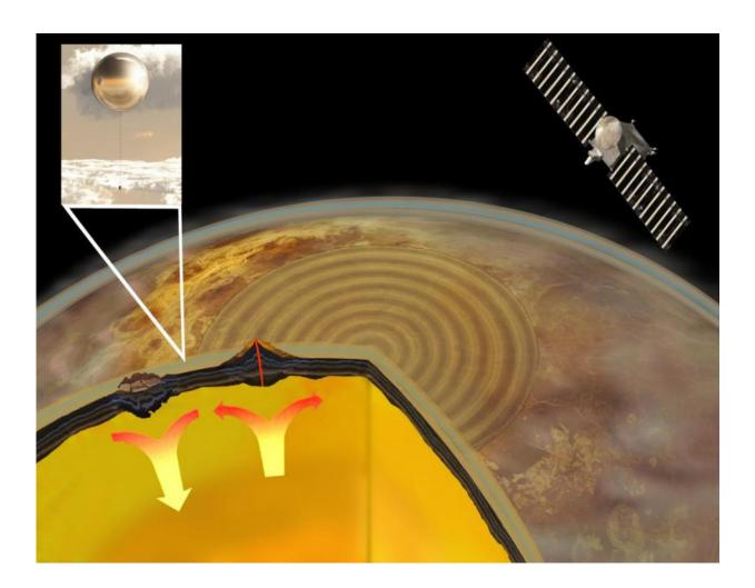
Seismic waves radiating from a Venus quake propagate as Rayleigh waves in the Venus surface layers and generate infrasonic waves traveling upwards through the dense Venus atmosphere. These low frequency sound waves can be detected by a balloon (upper left) floating within the Venus clouds at an altitude of 55 km where temperatures are similar to those on the Earth's surface. As the infrasonic
