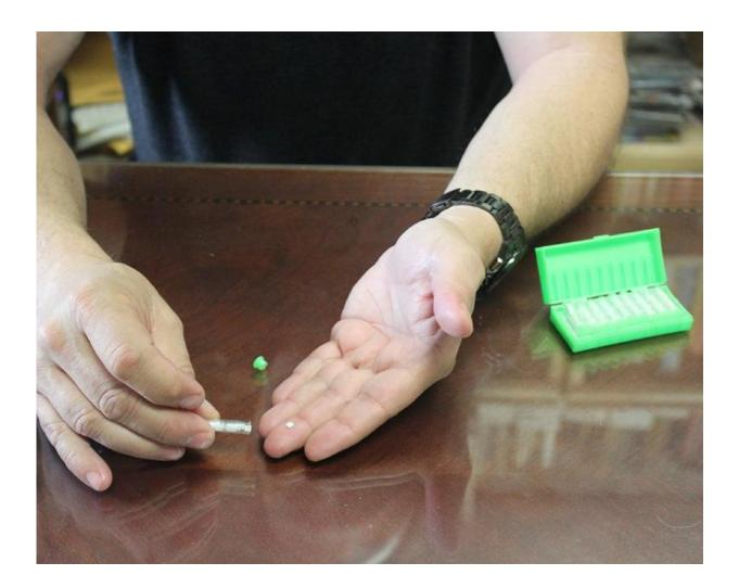
A detector absorbs the energy of gamma radiation within defects in the crystal structure. When heated to 300 to 400 degrees Centigrade, the crystal releases the energy as luminescence that can be quantified. Credit: University of South Carolina
