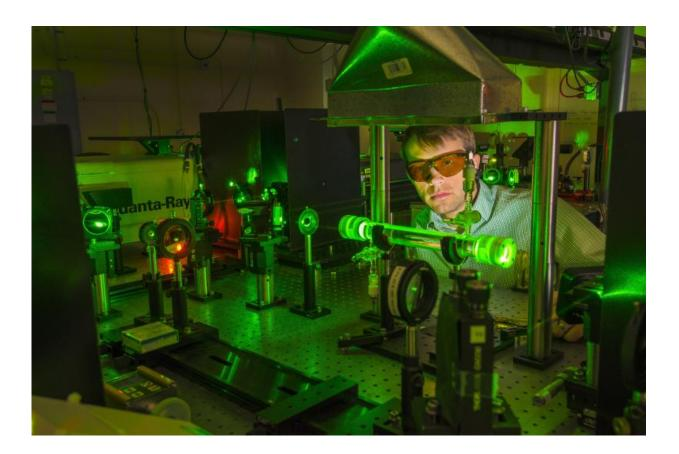
Sandia National Laboratories researcher Daniel Guildenbecher and colleagues have developed 3-D measurement techniques based on digital in-line holography to understand the generation and behavior of burning droplets of fuel from such incidents as transportation crashes. In his lab, he simulates a four-wave mixing cell to generate phase-conjugate light, one of the techniques used. Credit: Randy Montoya
