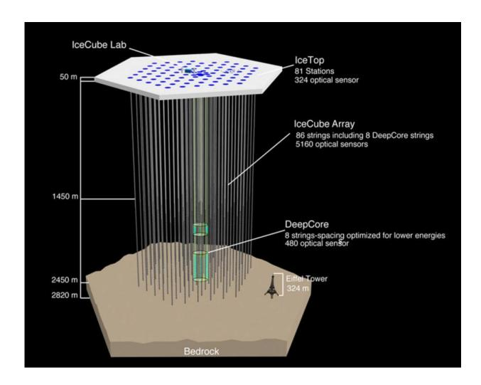
IceCube is comprised of a cubic kilometer of ice, which is densely packed with optical modules. The detector is located deep below the surface - – it starts  $1\frac{1}{2}$  km below the ice and ends at the bottom at a depth of  $2\frac{1}{2}$  km. The instruments in the detector are comprised of 86 cables each with 60 digital Optical Modules (extremely sensitive light sensors). Credit: IceCube Collaboration
