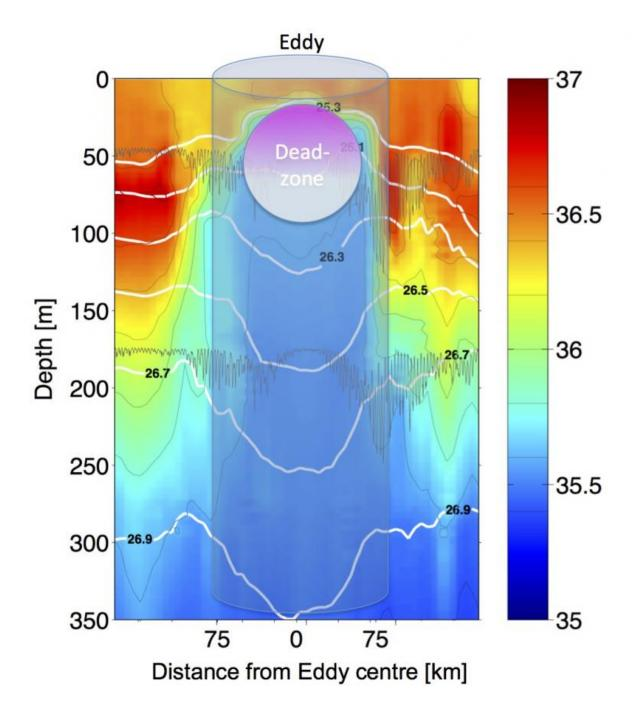
This plot shows a salinity section of the upper 350 metres of sea water observed across an eddy passing through the Cape Verde Ocean Observatory mooring. As the water in the eddy originates from the African Coast it is much lower in salinity than the surrounding water. The white contours represent levels of constant sea-water density, which bend downward towards the centre of the eddy, indicating rotation. The dead-zone (represented by the magenta circle)
