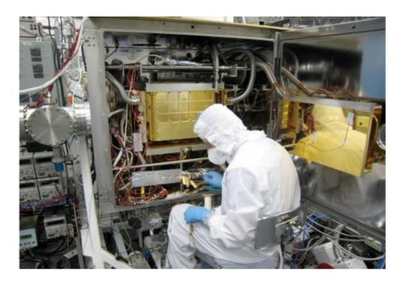
A Sample Analysis at Mars (SAM) team member at NASA Goddard prepares the SAM testbed for an experiment. This test copy of the SAM suite of instruments is inside a chamber that, when closed, can model the pressure and temperature environment that SAM sees inside Curiosity on Mars. Credit: NASA
