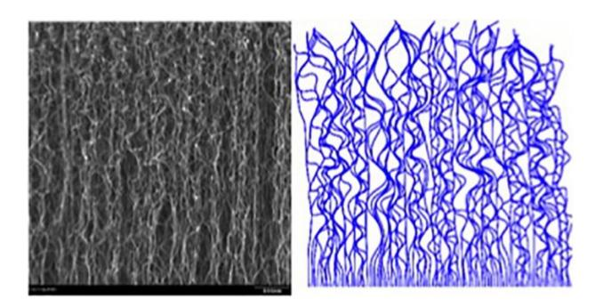
On the left is a scanning electron micrograph of a carbon nanotube forest. The figure on the right is a numerically simulated CNT forest. Credit: Matt Maschmann
