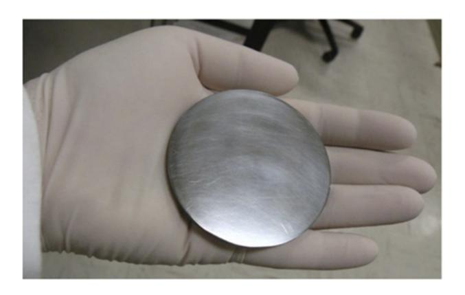
This thermoelectric material called skutterudite can be used for power generation. Credit: NASA/JPL-Caltech
