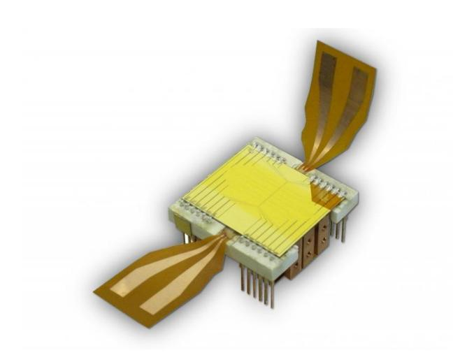
Atom chip for capturing and cooling clouds of atoms. Credit: TU Wien
