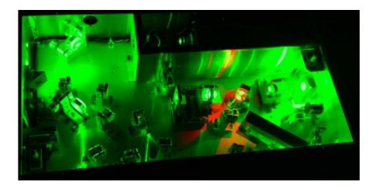
Extremely short pulses of red light (quadrillionths of a second) are generated by a titanium-sapphire laser, and then converted into terahertz light. The red glowing component in the photograph shown above is the titanium-sapphire crystal, surrounded by mirrors used in the laser. Credit: Brandon Carroll/Caltech
