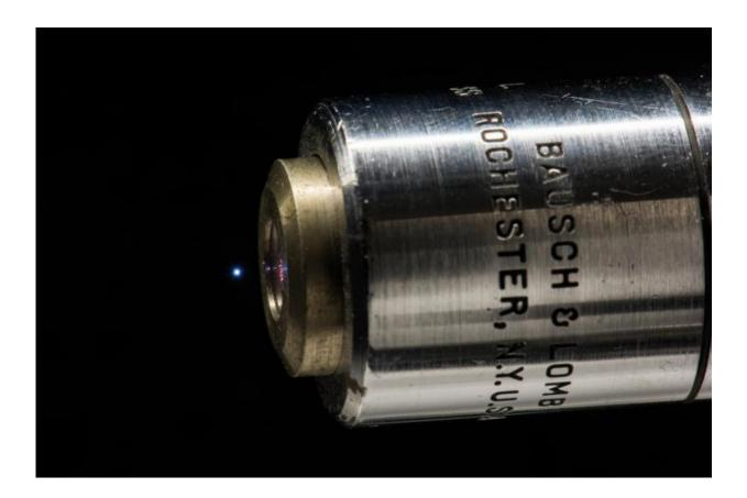
A microplasma is created by focusing intense laser pulses in ambient air with a microscope objective in the lab of University of Rochester Institute of Optics Ph.D. student Fabrizio Buccheri and his advisor, Professor Xi-Cheng Zhang. Besides visible light, the microplasma emits electromagnetic pulses at terahertz frequencies that can be used to detect complex molecules, such as explosives and drugs. Credit: J. Adam Fenster / University of Rochester
