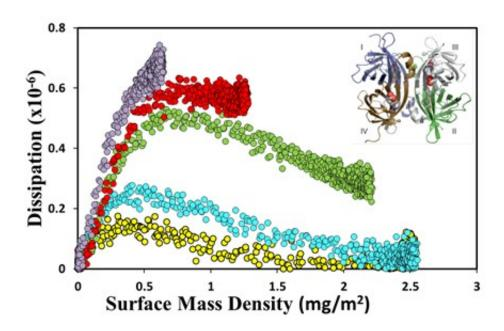
Representative image of correlation between quartz crystal microbalance with dissipation data with spectroscopic ellipsometry.
