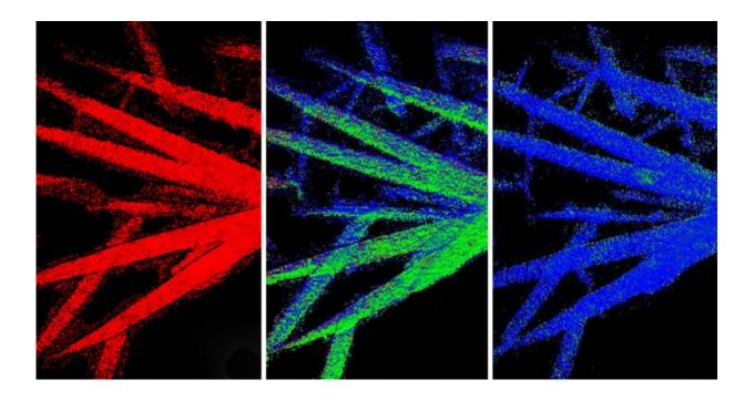
Chemical phase map shows how the electrochemical discharge of iron fluoride microwires proceeded from 0 percent discharge (left), to 50 percent (middle), to 95 percent (right). Credit: Linsen Li
