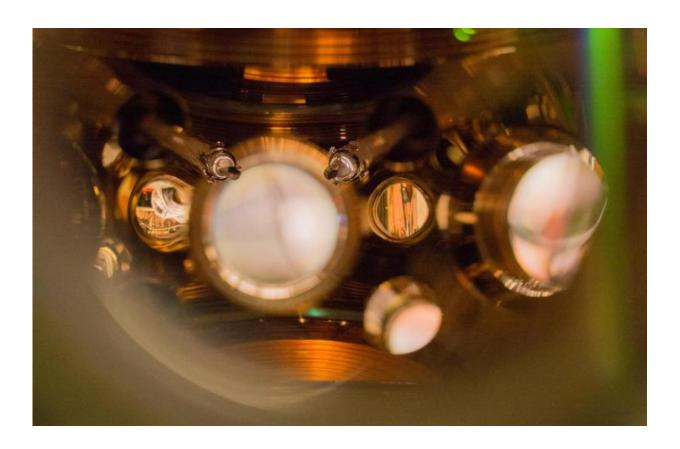
JILA's strontium lattice atomic clock now performs betterthan ever because scientists literally "take thetemperature" of the atoms' environment. Two specializedthermometers, calibrated by NIST researchers and visible in the center of the photo, are inserted into the vacuum chamber containing a cloud of ultracoldstrontium atoms confined by lasers. Credit: Marti/JILA
