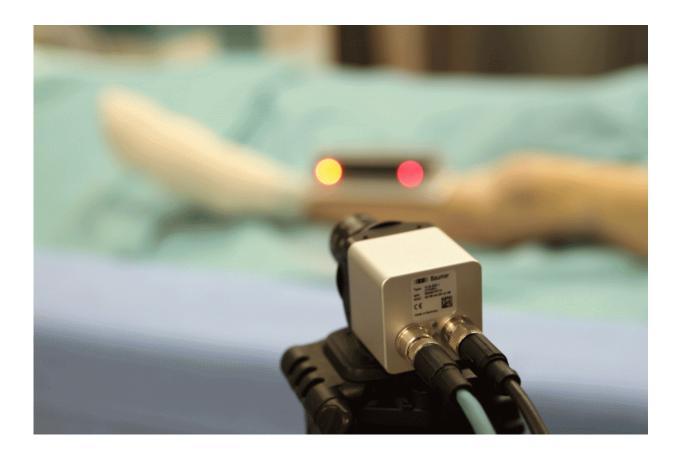
Measuring system for determining leg length. Credit: Fraunhofer IWU
