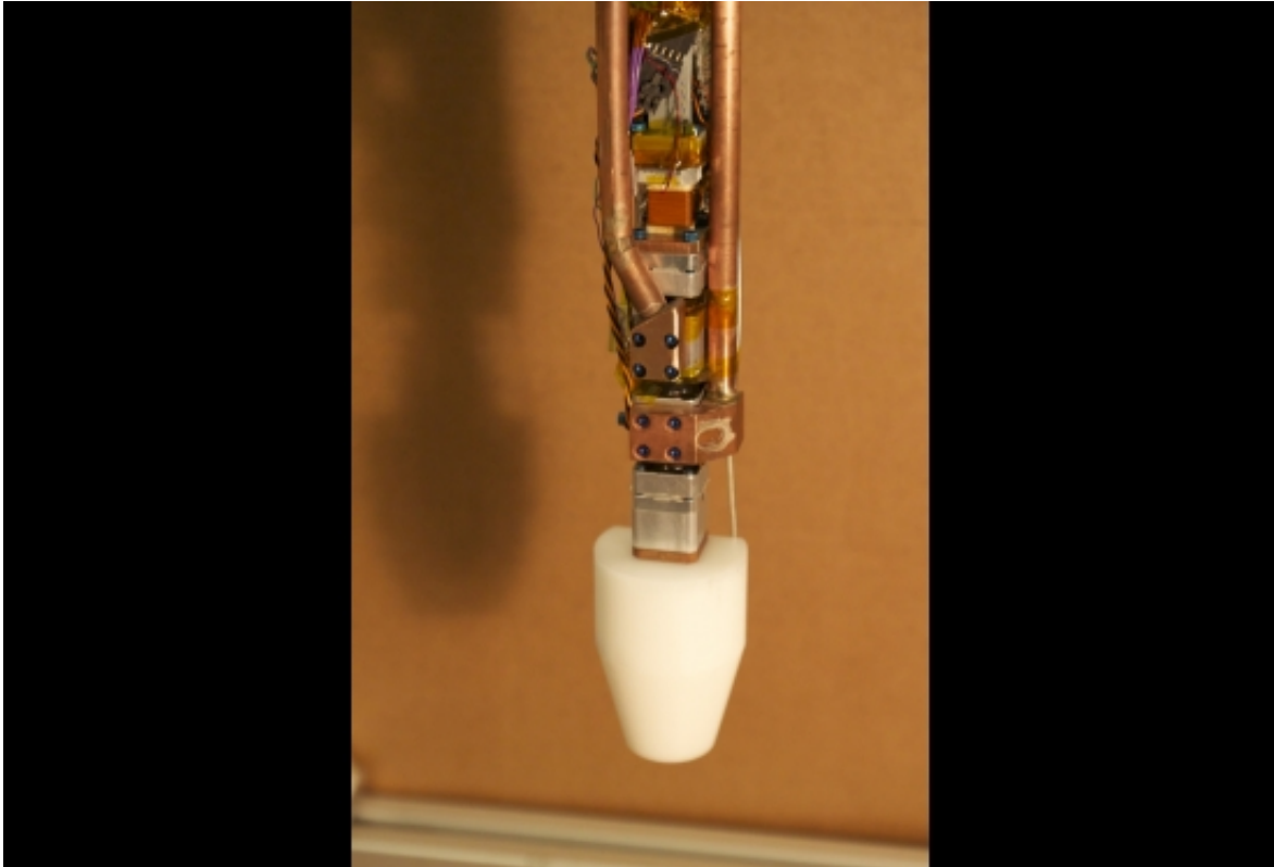
The gas lines and trapping cell can be seen in the 51-mm-wide waveguide insert. Credit: UCSB
