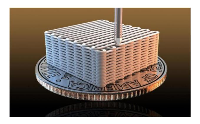
Lawrence Livermore researchers have made graphene aerogel microlattices with an engineered architecture via a 3D printing technique known as direct ink writing. Credit: Ryan Chen/LLNL
