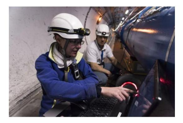
Engineers Aline Piguiet and Markus Albert take X-rays of the shorted superconducting dipole in sector 3-4 in the LHC tunnel . Credit: Maximilien Brice/CERN
