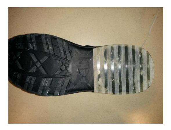
The heel of this prototype winter shoe is made from a rubbery plastic embedded with tens of thousands of tiny glass fibers that protrude out of the rubber like microscopic studs to grip the ice. Credit: Reza Rizvi, Yue Li, and Sharon Ravindran/ Toronto Rehabilitation Institute
