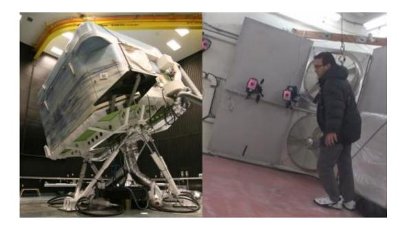
The team is testing the composite material with winter shoes by asking volunteers wearing the shoes to walk up and down an ice-covered inclined floor. The inclined floor is part of WinterLab, shown on the left, which is a self-contained tiltable room that is part of the Challenging Environment Assessment Lab at the Toronto Rehabilitation Institute. Credit: Reza Rizvi, Yue Li, and Sharon Ravindran/ Toronto Rehabilitation Institute
