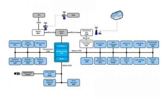
A simple two-tier architecture drastically reduces complexity. All driving and safety relevant functions run in one layer, while comfort functions, as well as communications between system, driver and internet are located in the other. Essential for security is that the components have only read access to vehicle data. Only in clearly defined cases for predefined functions the central ECU grants write access. Credit: TUM
