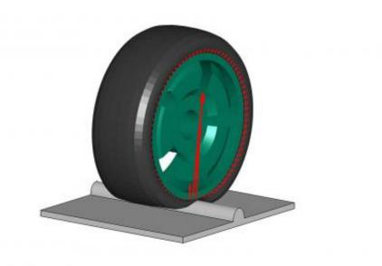
CDTire/3D tire simulation while rolling over an obstacle. Credit: Fraunhofer ITWM
