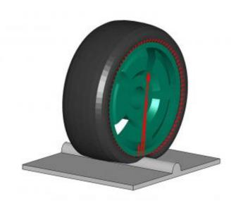
CDTire/3D tire simulation while rolling over an obstacle. Credit: Fraunhofer ITWM
