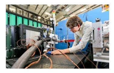
To observe the effects of heat on refrigerants, ORNL researcher Patrick Geoghegan used the High Flux Isotope Reactor to capture undistorted neutron images.
